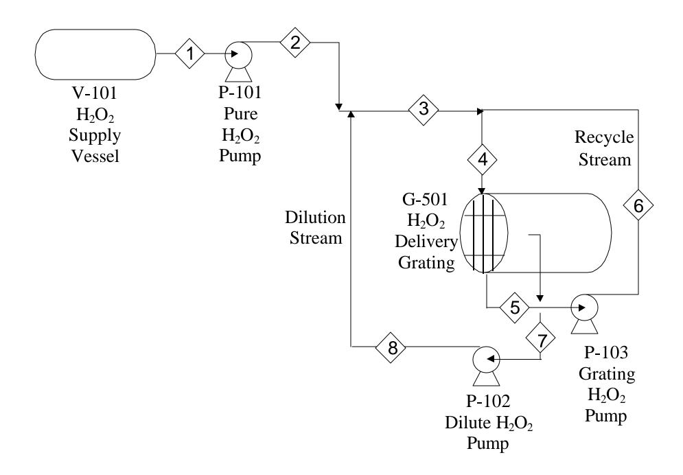
**Figure 2: Process Flow Diagram for Zebra Mussel Chemical Removal**
