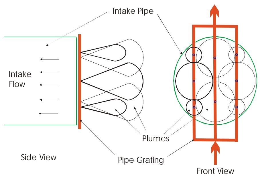
Figure 1: Optimum Jet Dispersion
