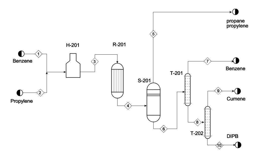
Figure 1: Preliminary Process Flow Diagram for Cumene Production
